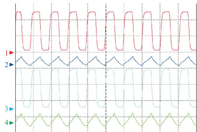
**Fig. 12.** Signal waveforms (500 ns/div) of voltages  $U_{flyDC+}$  (2 V/div) and  $U_{out-}$  (50 mV/div) under different load currents: 1, 2 – 147 mA; 3, 4 – 239 mA
