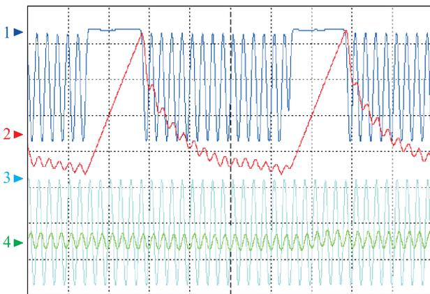
**Fig. 6.** Signal waveforms (2  $\mu\text{s}/\text{div}$ ) of voltages  $U_{flyDC-}$  (1 V/div) and  $U_{out-}$  (20 mV/div) under different load currents: 1, 2 – 50 mA; 3, 4 – 100 mA
