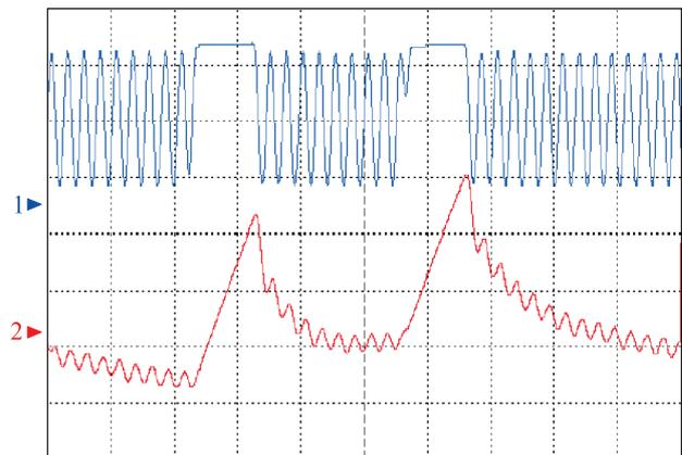
**Fig. 8.** Signal waveforms (2  $\mu\text{s}/\text{div}$ ) of voltages: 1 –  $U_{flyDC+}$  (2 V/div); 2 –  $U_{out-}$  (50 mV/div) under load current of 100 mA
