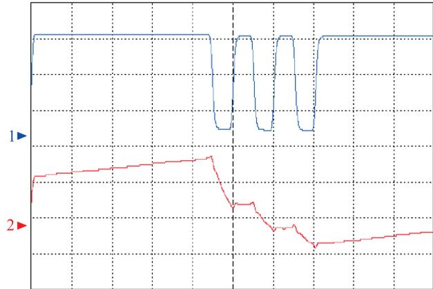
**Fig. 7.** Signal waveforms (500 ns/div) of voltages: 1 –  $U_{flyDC+}$  (2 V/div); 2 –  $U_{out-}$  (50 mV/div) under load current of 15 mA
