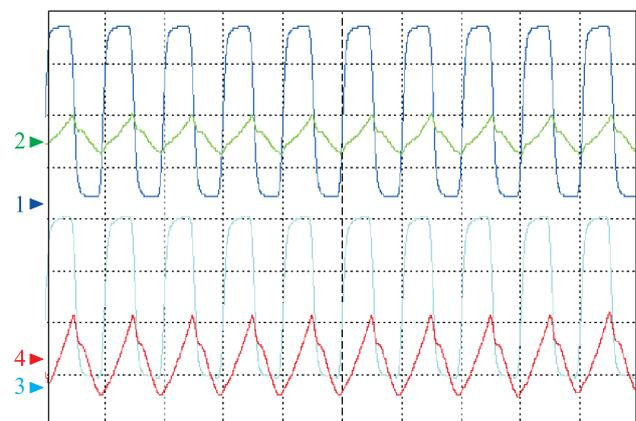
**Fig. 4.** Signal waveforms (500 ns/div) of voltages  $U_{flyDC+}$  (1 V/div) and  $U_{out-}$  (20 mV/div) under different load currents: 1, 2 – 100 mA; 3, 4 – 250 mA
