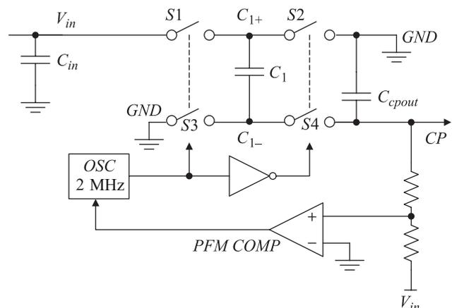
Fig. 1. Voltage inverting principle [8]
