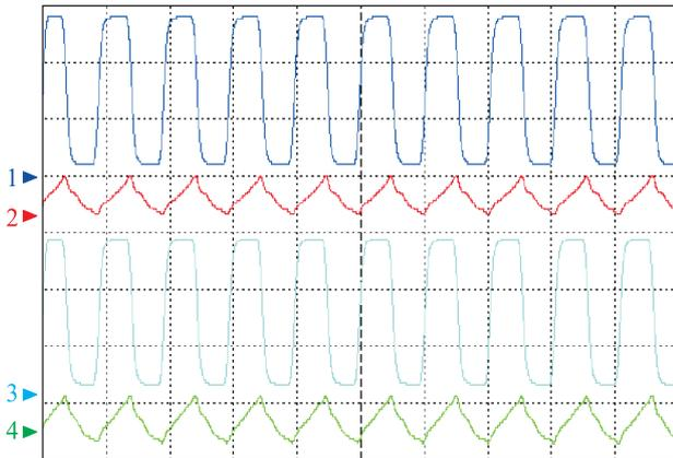
**Fig. 9.** Signal waveforms (500 ns/div) of voltages  $U_{flyDC+}$  (2 V/div) and  $U_{out-}$  (50 mV/div) under different load currents: 1, 2 – 153 mA; 3, 4 – 220 mA
