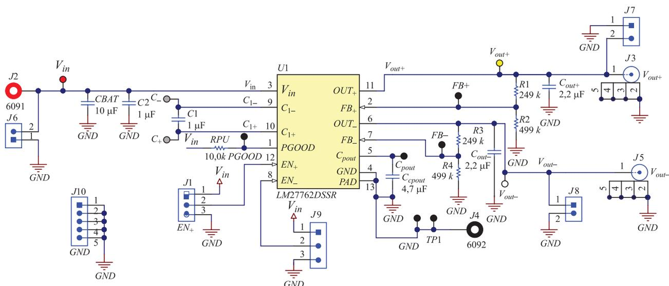
Fig. 2. Schematic of *LM27762EVM* module PCB [9]
