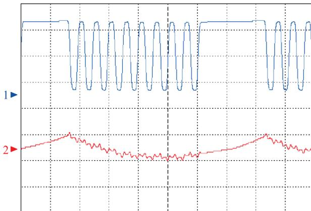
**Fig. 10.** Signal waveforms (1  $\mu$ s/div) of voltages  $U_{flyDC-}$  (2 V/div) and  $U_{out-}$  (20 mV/div) under load current of 90 mA
