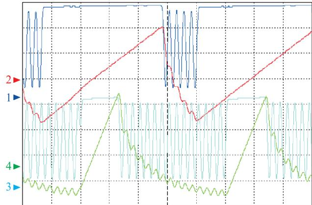
**Fig. 3.** Signal waveforms (2 μs/div) of voltages  $U_{flyDC+}$  (1 V/div) and  $U_{out-}$  (20 mV/div) under different load currents: 1, 2 – 15 mA; 3, 4 – 50 mA
