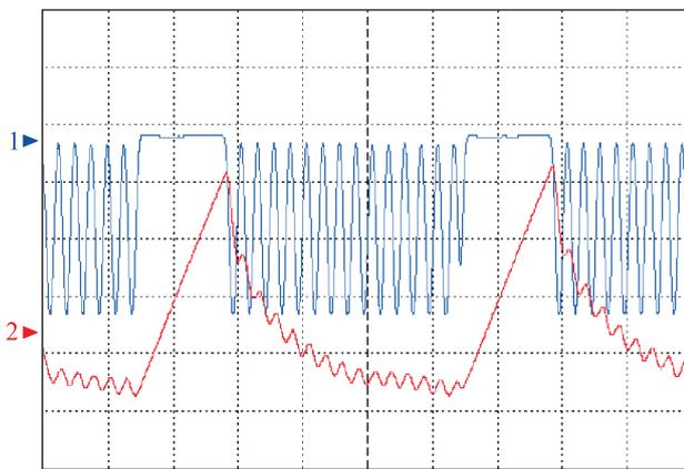
**Fig. 5.** Signal waveforms (2  $\mu\text{s}/\text{div}$ ) of voltages: 1 –  $U_{flyDC+}$  (1 V/div); 2 –  $U_{out-}$  (20 mV/div) under load current of 50 mA
