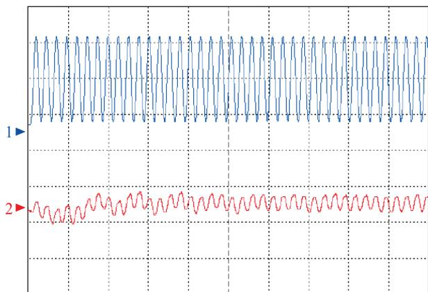
**Fig. 11.** Signal waveforms (2  $\mu$ s/div) of voltages  $U_{flyDC-}$  (2 V/div) and  $U_{out-}$  (20 mV/div) under load current of 157 mA
