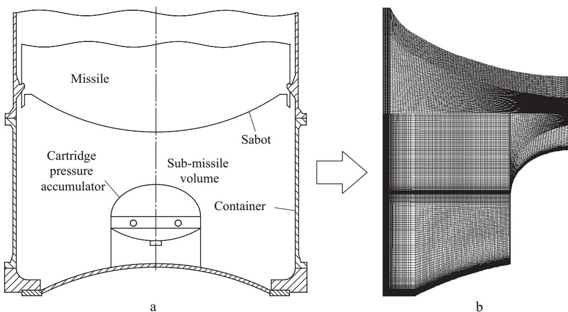
Fig. 1. Grid motel generation stages: a – sabot layout; b – grid model
