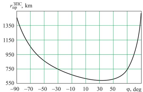
Fig. 5. Angular dependence of penetration range for manoeuvre and tail-chase engagement
