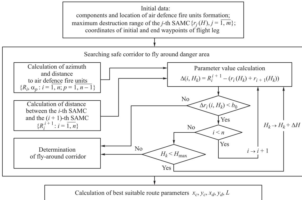
**Fig. 3.** Block diagram showing the algorithm for calculating the elements of the best suitable route to fly around the kill zone controlled by a SAMC formation
