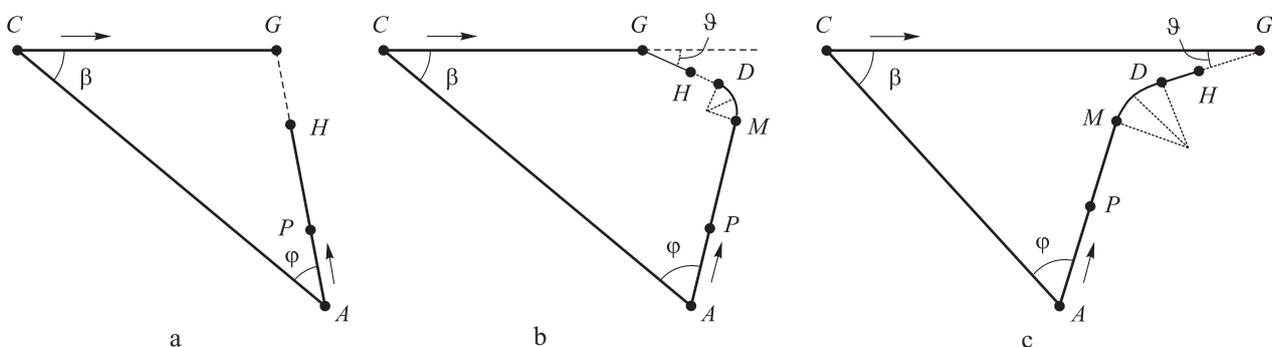
**Fig. 4.** Aircraft route patterns in case of direct interception (a), in case of manoeuvre and head-on engagement (b) in case of manoeuvre and tail-chase engagement (c):  $A$  – aircraft flight origin;  $C$  – initial target location;  $P$  – balanced flight leg origin;  $CG$  – target penetration range;  $MD$  – flight leg with aircraft manoeuvre;  $H$  – aircraft position at missile launch;  $G$  – position of target when hit by air-to-air missile
