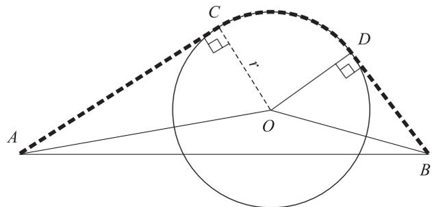
**Fig. 2.** Geometry of the shortest curve to fly around a danger area
