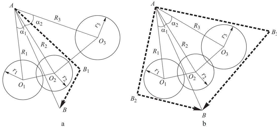
**Fig. 1.** Variants of safe corridors to fly around a kill zone in the area of joint responsibility if there is a gap (a) or no gap (b)
