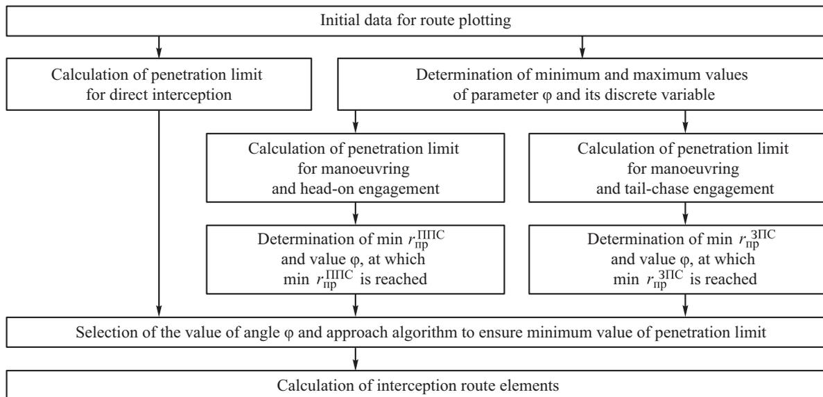
Fig. 6. Block diagram of the route elements calculation algorithm to minimize the air target penetration range
