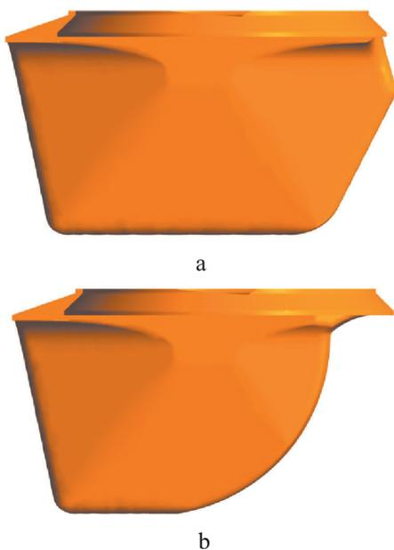
Fig. 1. JV airfoil portion profile at the beginning (a) and at the end (b) of SPRE operation
