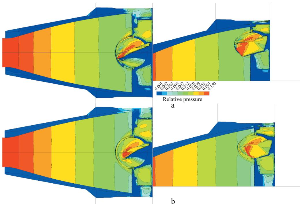
**Fig. 3.** Distribution of relative pressure in the structure: a – beginning of SPRE operation; b – end of SPRE operation
