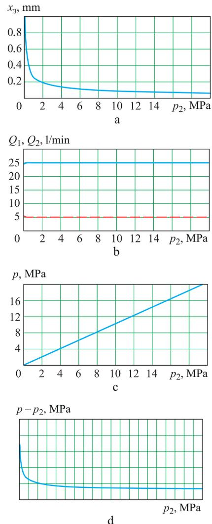
**Fig. 2.** Static performance characteristics of SFCV: a – dependence of spool position  $x_3$  on load pressure  $p_2$ ; b – dependence of volume flow rates  $Q_1$  and  $Q_2$  supplied through SFCV on load pressure; c – dependence of SFCV inlet pressure  $p$  on load pressure  $p_2$ ; d – dependence of SFCV pressure differential on load pressure
