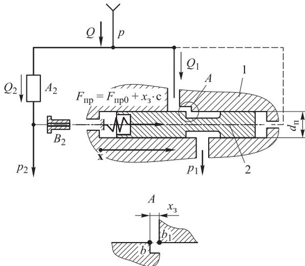
**Fig. 1.** Analytical diagram of the three-port SFCV static model: 1 – sleeve; 2 – spool; A – detail;  $\mathbf{x}$  – coordinate vector
