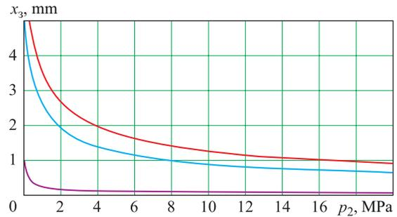
**Fig. 4.** Dependence of spool  $x_3$  positions on load pressure for: — sharp-edged spool; — spool with two 45° grooves; — spool with two 30° grooves
