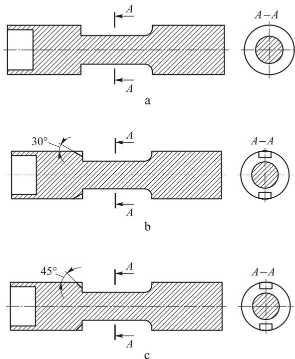
**Fig. 3.** Several spool geometry options: a – spool with sharp edge (No. 1); b – spool with two 45° grooves (No. 2); c – spool with two 30° grooves (No. 3)
