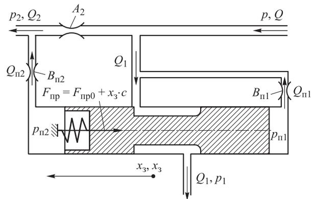
**Fig. 5.** Analytical diagram of the three-port SFCV dynamic model
