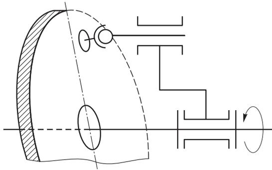
Fig. 1. Kinematic diagram of piston mechanism
