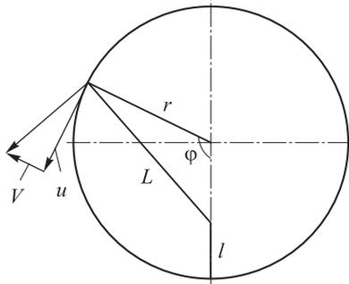
**Fig. 3.** Diagram of velocities of arbitrary point on the surface:
