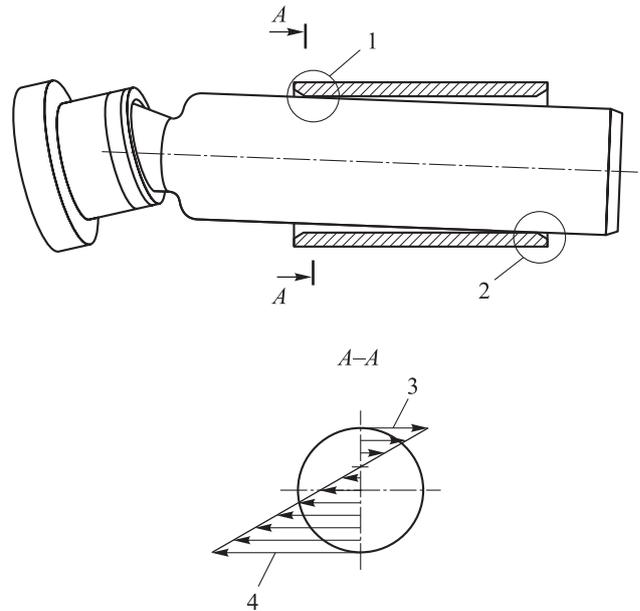
Fig. 2. Relative tangential velocity of piston on the outer edge:
