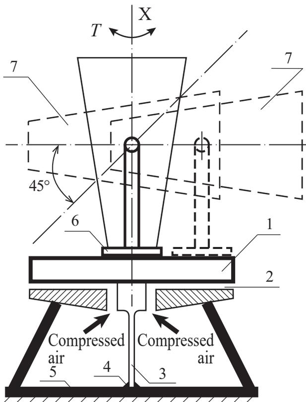
**Fig. 1.** Diagram of unifilar test bench with a possibility to horizontally displace the tested item:
