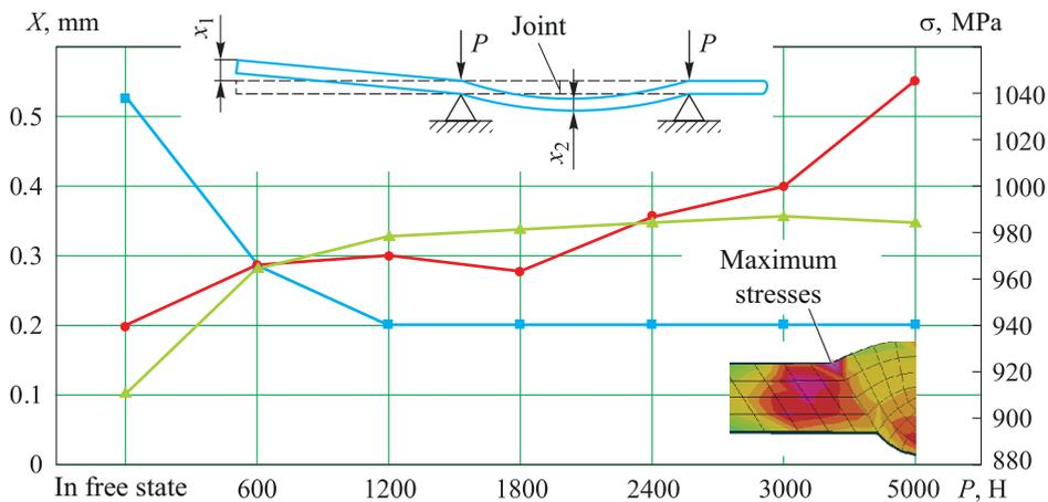
Fig. 4. Change of the maximum residual stresses and deformations as a function of  $P$  :
