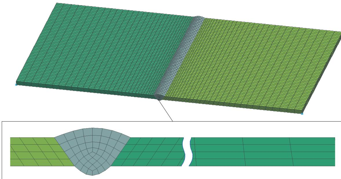
Fig. 3. Mesh for thermal and mechanical problem solution
