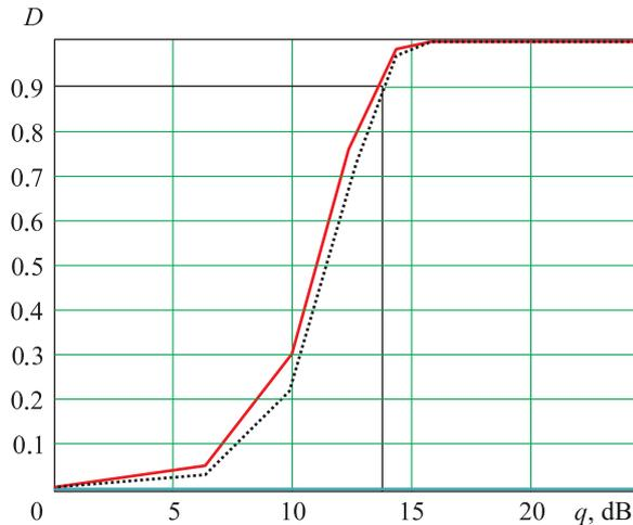
**Fig. 2.** Detection curves of incoherent pulse burst (with inter-pulse correlation coefficient  $r = 0$ ) after incoherent integration of pulses (—), under processing as per the proposed algorithm with account of inter-period Doppler phase advance (.....), and after coherent integration of pulses (—)
