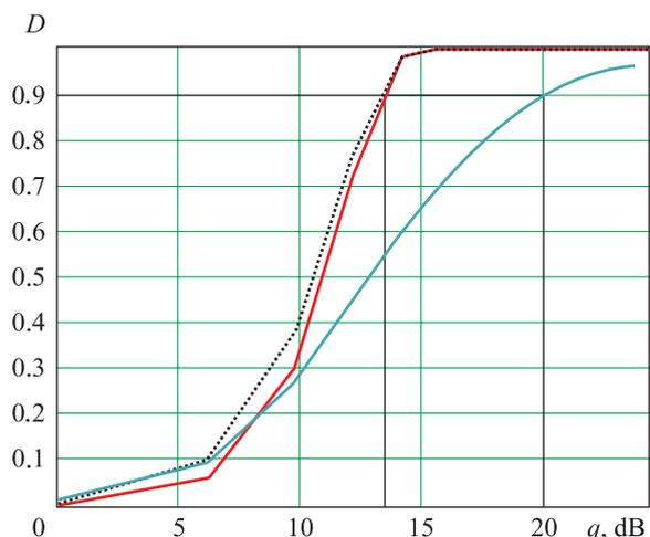
**Fig. 5.** Detection curves of partly coherent pulse burst consisting of four incoherent sub-bursts (with inter-sub-burst correlation coefficient  $r = 0$ ) after their incoherent integration (—), under processing as per the proposed algorithm with account of inter-period Doppler phase advance (.....), and after their coherent integration (—)
