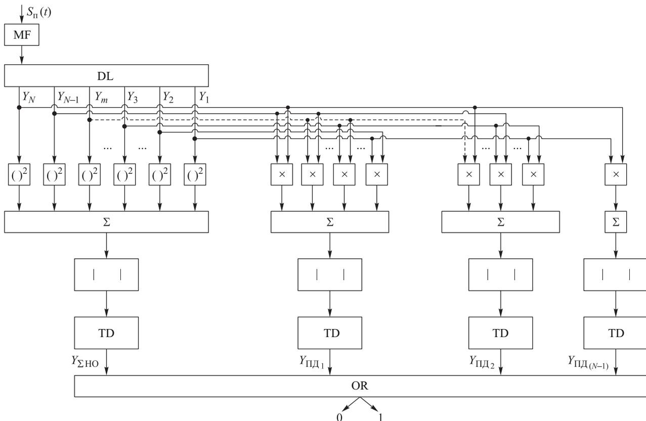
Fig. 1. Block diagram of algorithm for receiving a pulse burst with account of inter-period Doppler phase advance
