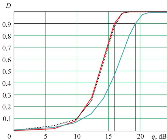
**Fig. 3.** Detection curves of partly coherent pulse burst (with inter-pulse correlation coefficient  $r = 0.35$ ) after incoherent integration of pulses (—), under processing as per the proposed algorithm with account of inter-period Doppler phase advance (.....), and after coherent integration of pulses (—)
