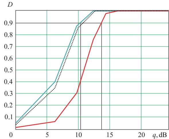
**Fig. 4.** Detection curves of coherent pulse burst (with correlation coefficient  $r = 1$ ) after incoherent integration of pulses (—), under processing as per the proposed algorithm with account of inter-period Doppler phase advance (.....), and after coherent integration of pulses (—)
