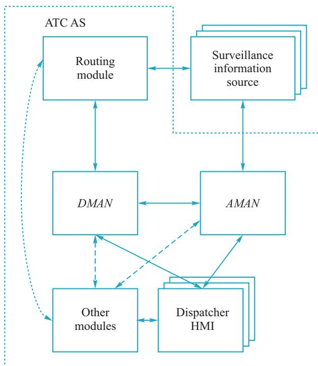
Fig. 1. *DMAN* communication with other system modules
