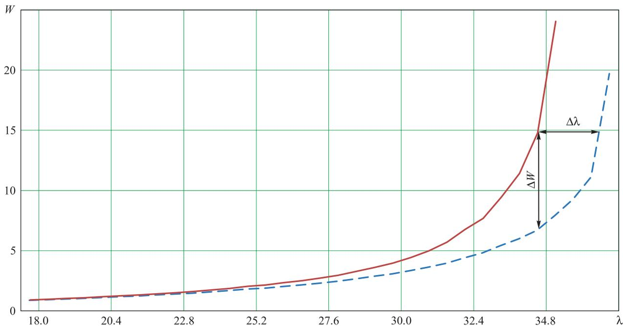
Fig. 2. Dependency between the average departure delay time and the density of departures for prioritized (— —) and non-optimized (—) queues
