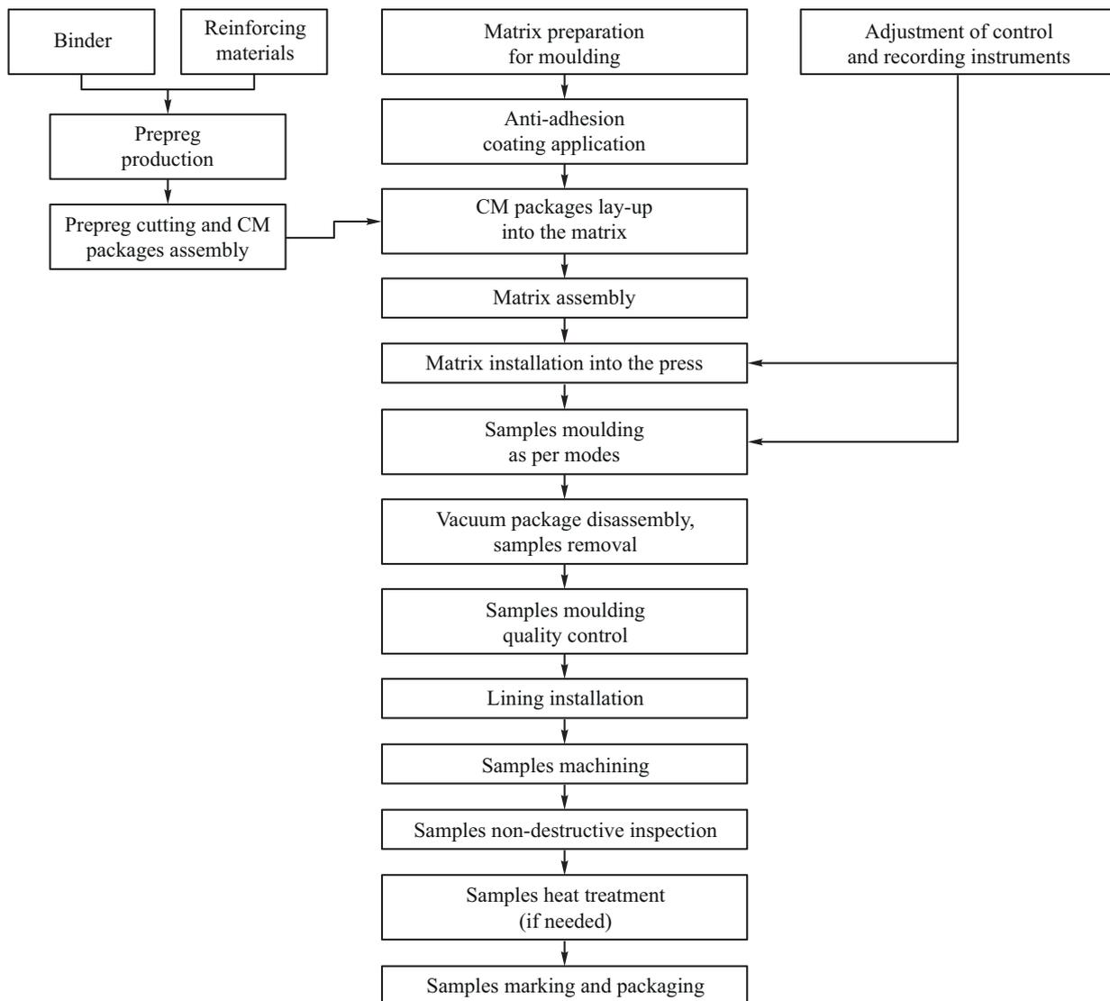
Fig. 1. Sample manufacturing process, series 11 and 12, with *Epolam 2092* binder
