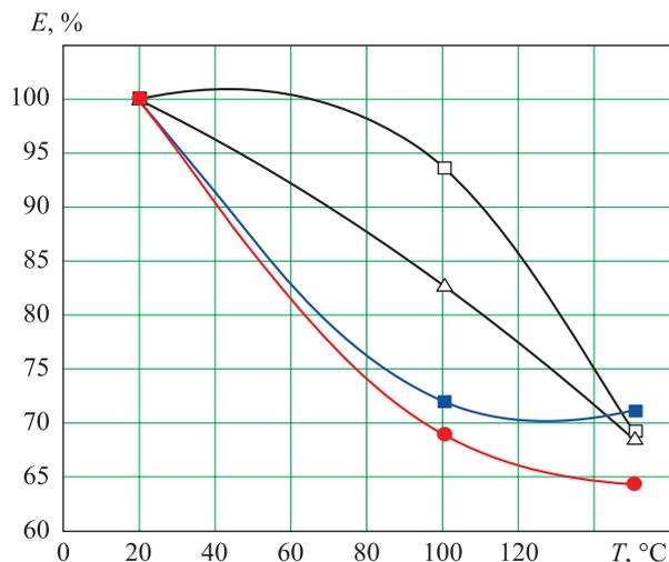
**Fig. 7.** Relative variation of  $E$  modulus depending on tension temperature, sample numbers:
