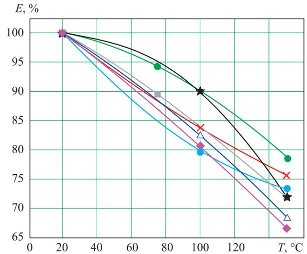
Fig. 5. Relative variation of  $E$  modulus depending on compression temperature, sample numbers:
