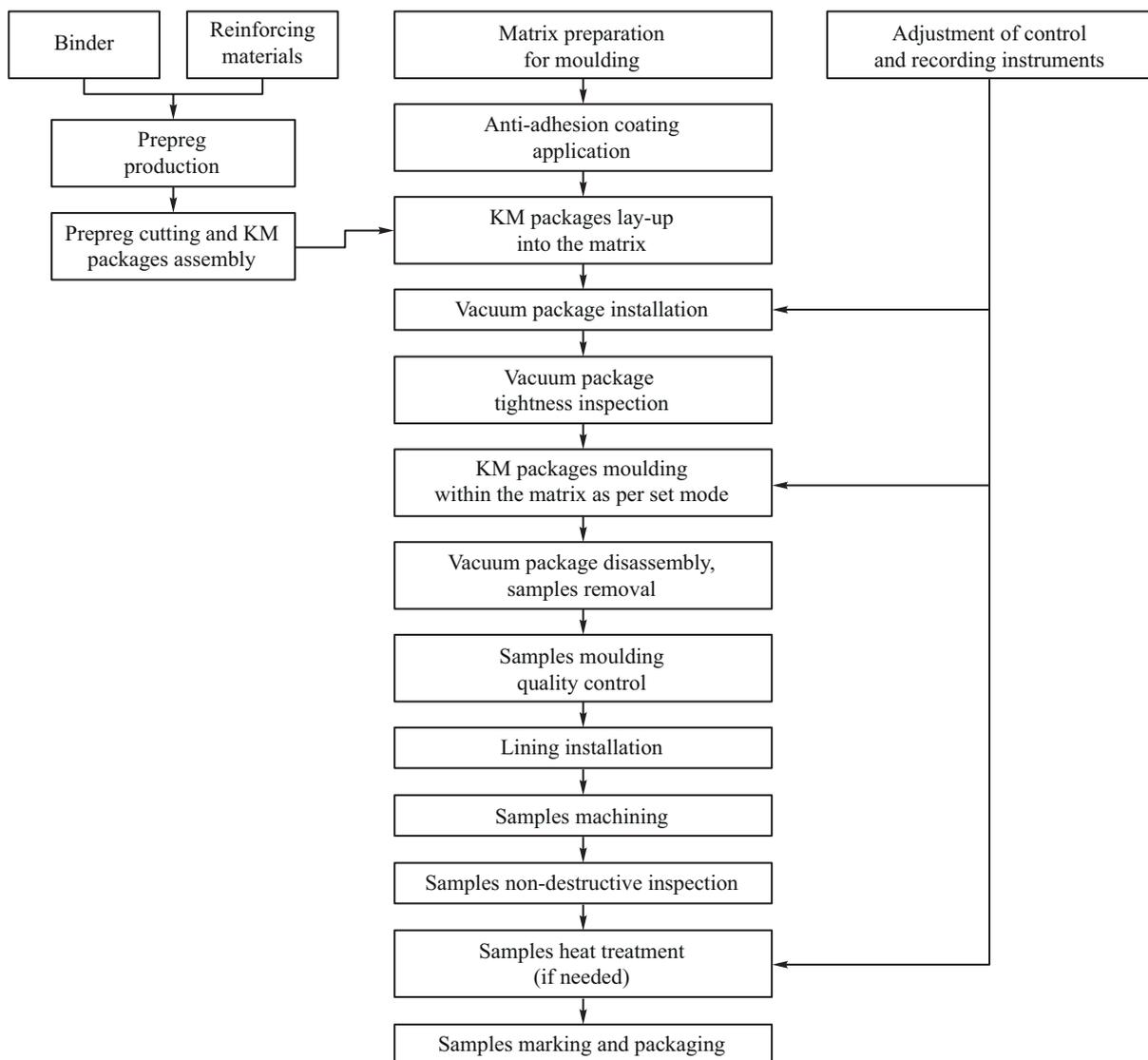
Fig. 2. Sample manufacturing process, series 1–4, 13, 14, with “Alumoepoxy” binder
