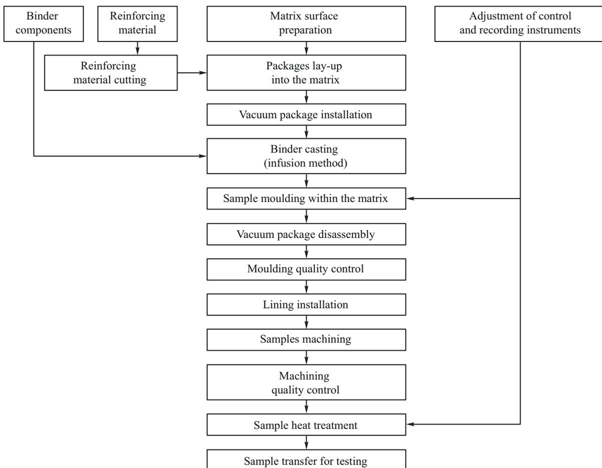
Fig. 3. Sample manufacturing process, series 5–10, with CR-122 binder
