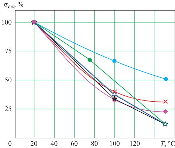
Fig. 4. Relative variation of  $\sigma_{cjk}$  depending on compression temperature, sample numbers:
