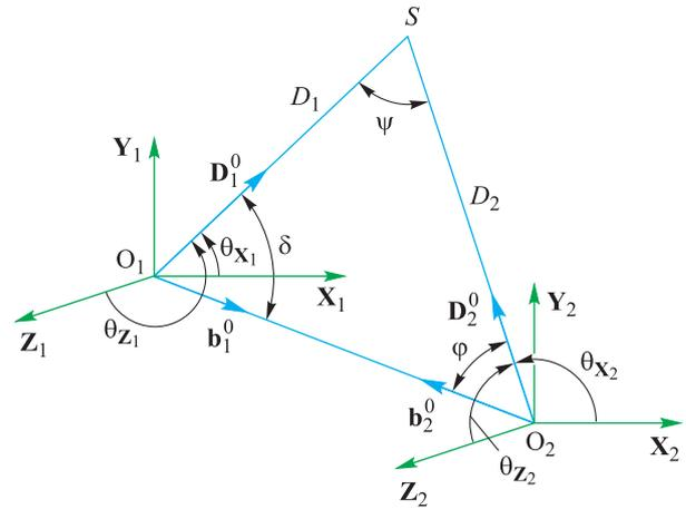
Fig. 3. Determination of object coordinates using two MFs
