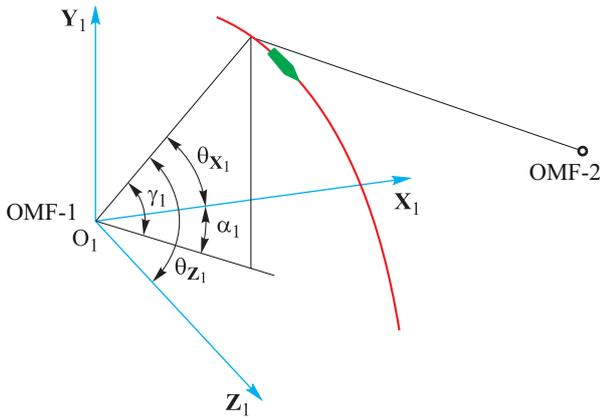
Fig. 2. Transition from azimuth and elevation angle to measurements in the form of direction cosines
