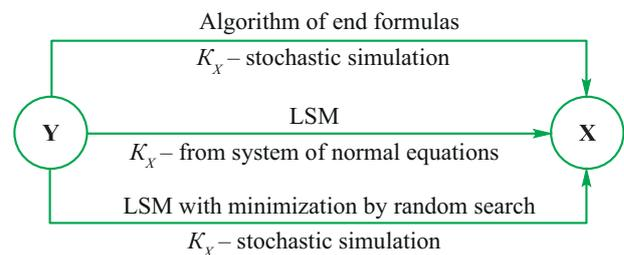
Fig. 1. Method of trajectory determination accuracy calculation using a minimum set of measurements
