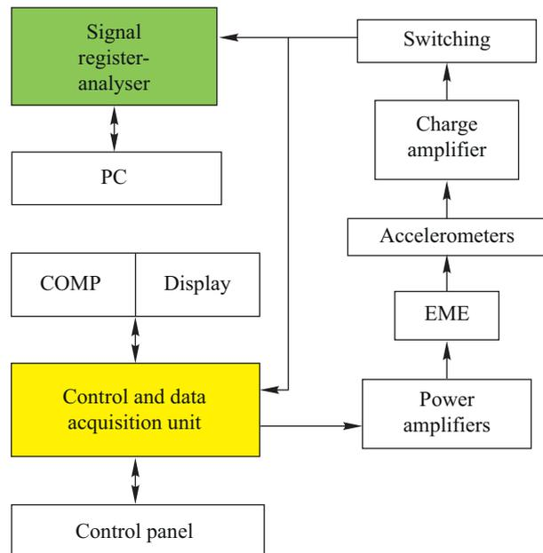
Fig. 5. The block diagram of the experiment: EME – an electromechanical oscillation exciter
