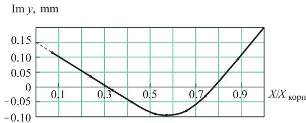
Fig. 4. Normal shape of the body first bending mode
