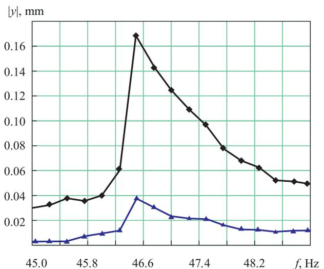
**Fig. 6.** Amplitude-frequency response of the body oscillations in  $Oxy$  (◆) and  $Oxz$  (▲) planes
