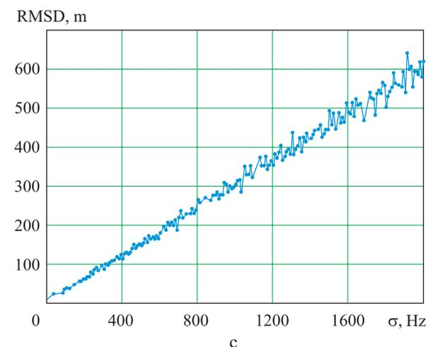
**Fig. 2.** RMSD dependences: on noise dispersion value a – deviations 40/60 kHz; b – deviations 300/500 kHz; c – deviations 3/5 MHz
