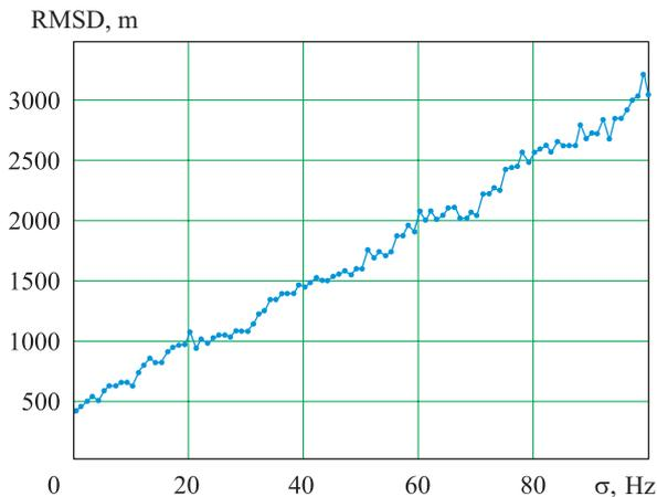
**Fig. 3.** RMSD dependence on noise dispersion value with reduced spacing of Doppler filters arrangement (deviations 40/60 kHz)
